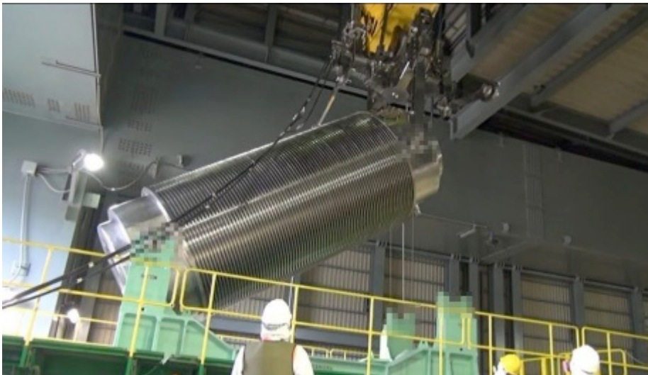
The cask holding the last used fuel assembly is moved to the shared storage pool. (Image: Tepco)
