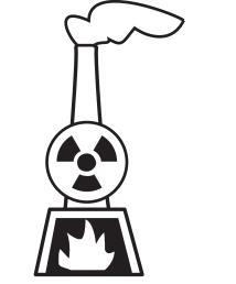
A RADWASTE INCINERATOR reduces the volume of combustible radioactive waste materials, yielding atmospheric releases and radioactive filters. Canada has one radwaste incinerator at Bruce.
