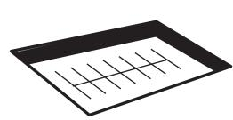
SPENT FUEL POOLS. When irradiated fuel is discharged from a reactor, it is stored under water. Spent fuel is far more radioactive than fresh fuel, due to new radioactive materials created inside the reactor. Water in the pool shields workers from lethal doses of radiation and prevents spent fuel from overheating as a result of radioactive decay.
