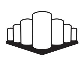
SPENT FUEL SILOS provide dry storage for spent fuel that has cooled off in a pool for seven years or more. By then, the radioactivity has declined enough that spent fuel can be cooled by air circulating through vents in concrete silos. However, since spent fuel remains hazardous for millions of years, pools and silos are only temporary storage measures.
