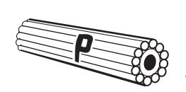
PLUTONIUM FUEL, or MOX ("mixed oxide") fuel, refers to a blend of uranium and plutonium oxides fabricated into new reactor fuel. Plutonium for MOX can come from dismantled nuclear warheads or reprocessed spent fuel. Unlike CANDU uranium fuel, plutonium fuel is a strategic material; it can be easily stolen or diverted, and used to make an atomic bomb.
